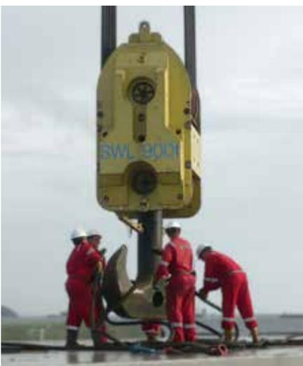
Vessel crew rigging the crane onboard MV Jumbo Javelin
